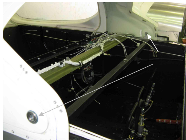
Canopy attachment bolts
