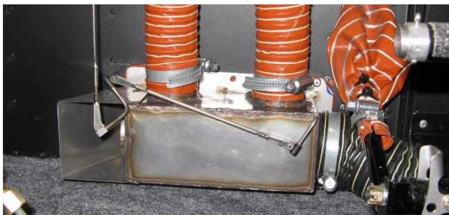
Fig. Heating mixing chamber
