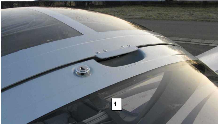
Fig. Cockpit canopy lock Cockpit is unlocked, when a latch is visible under the glass, otherwise it is locked. 1 - latch
