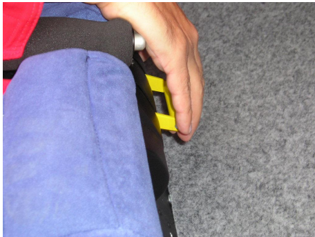
Picture: Parking brake OFF
