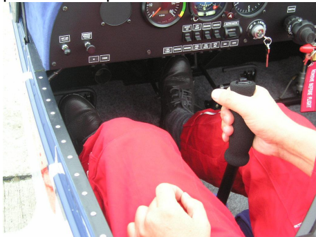
Picture: Deflection of right rudder pedal-the airplane turns to the right
