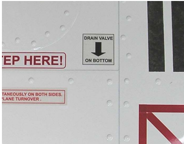
Picture: Placard-arrow marking location of drain valve
