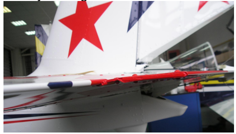
Picture: Trim tab deflected in Nose heavy position
