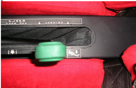
Picture: Green elevator trim tab control lever set to Tail heavy position
