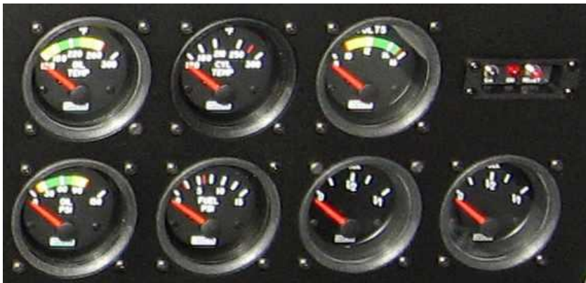
Picture: Detail view of engine analogue instruments-color markings
