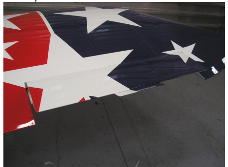
And corresponding up deflection of the right aileron (the left one deflected down)
