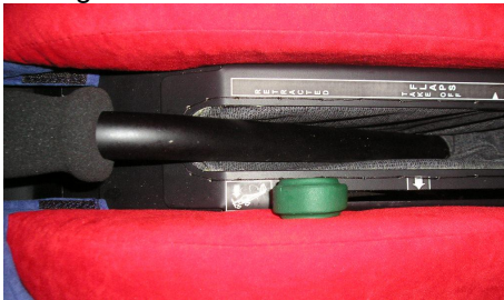
Picture: Green elevator trim tab control lever set to Nose heavy position
