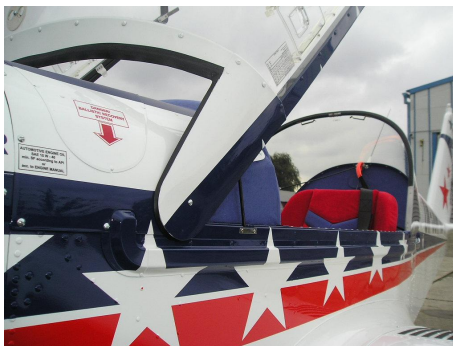
Picture: Ballistic system rear stabilizing cable guided on port side of fuselage to a rear suspension
