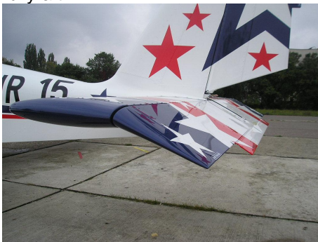
Elevator deflection with control stick fully forward
