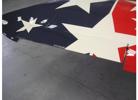
And corresponding up deflection of the left aileron (the right one deflected down)
