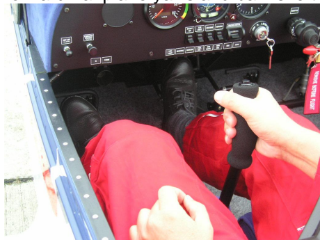
Picture: Right rudder pedal deflected forward— airplane yaws and banks right
