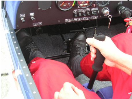
Picture: Deflection of left rudder pedal-the airplane turns to the left
