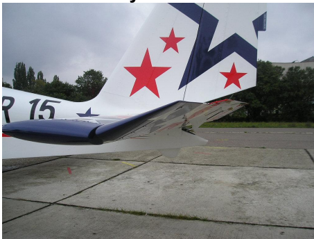
Elevator deflection with control stick fully aft
