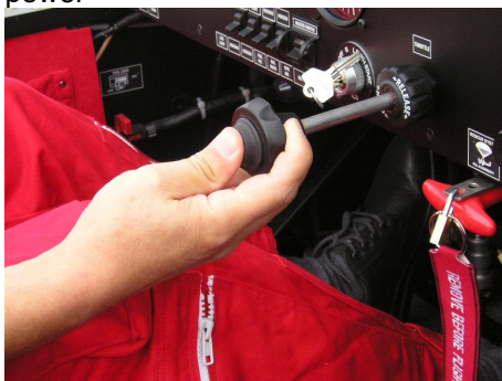
Picture: Rough setting of engine power
