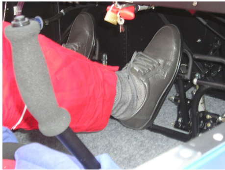
Picture: Foot during braking – tip-toe pushes on the toe-brake pedal
