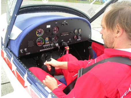
Picture: Stick deflected left – airplane banks and turns left
