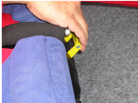
Picture: Parking brake ON
