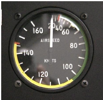
Picture: Airspeed indicator marked with color coded arcs
