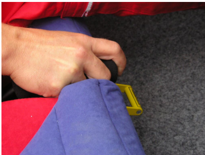
Picture: To extend flaps, first apply a little downward pressure on the handle and then press the button
