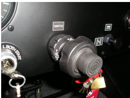
Picture: : Throttle lever set for max. power
