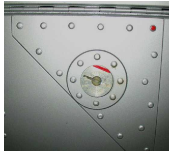
Picture: Fuel tank drain valve on the bottom of the each wing.
