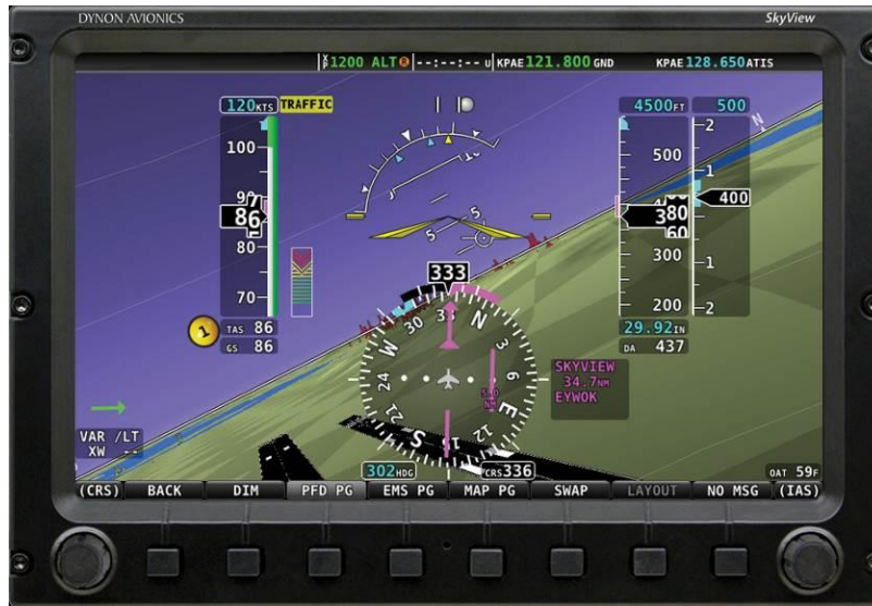
Figure 41 – SkyView Synthetic Vision View with Runways
