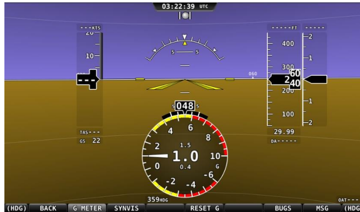
Figure 59 – G Meter on PFD
