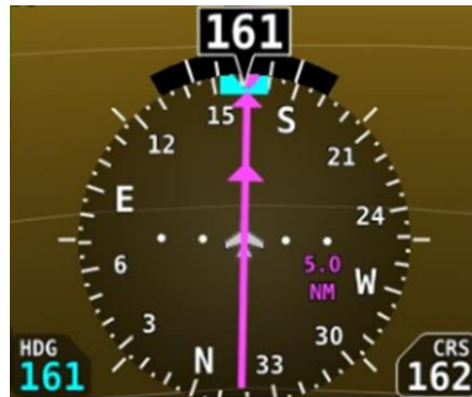
Figure 24 – HSI Example - GPS
