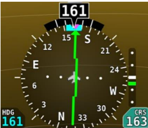
Figure 23 – HSI Example - Localizer
