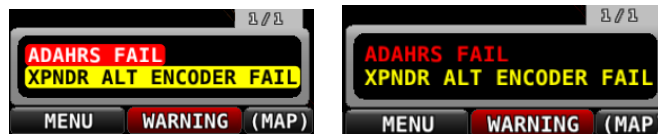
Figure 234 – Unacknowledged (left) and Acknowledged (right) Alarms
