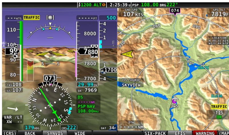
Figure 42 – SkyView Synthetic Vision Normal View
