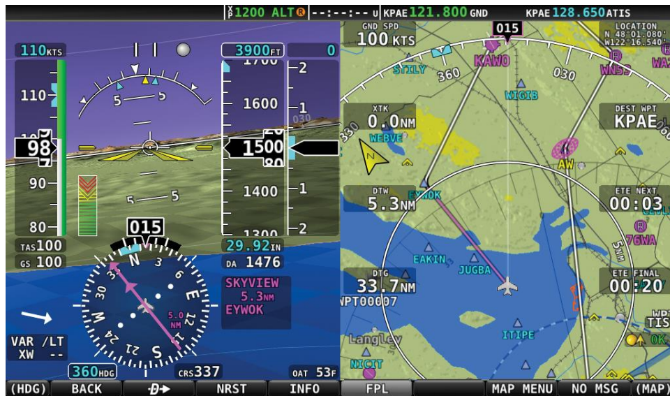
Figure 138 – Active Flight Plan: HSI and MAP Depictions
