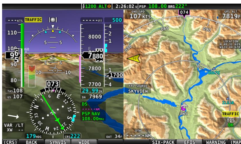
Figure 43 – SkyView Synthetic Vision Wide View
