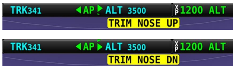
Figure 179 - Trim Nose Up and Down Alerts
